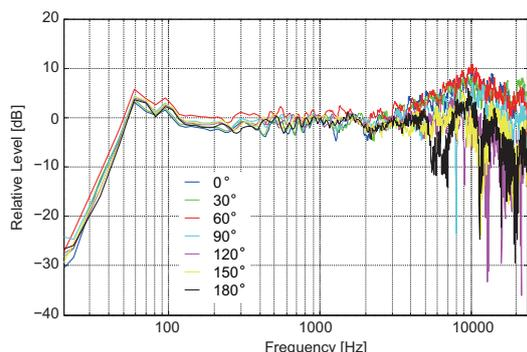
**Fig. 4:** Frequency response of #31 microphone. The rotated results for every 30 degrees are also plotted.
