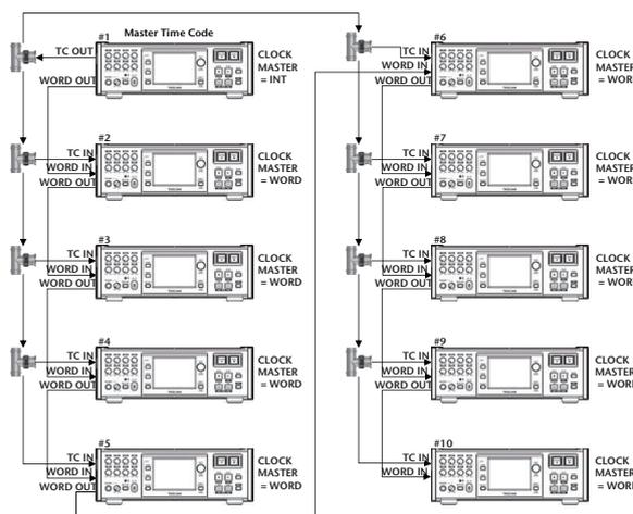
**Fig. 7:** Connection method of recorder for Time Code and Word Clock synchronization. Time code is distributed from the first machine to all others directly and the word clock was distributed by cascade connection.
