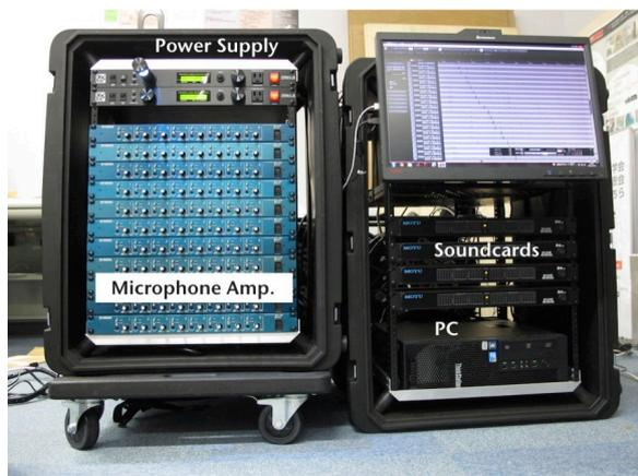
**Fig. 5:** Sound recording system based on PC and DAW (Nuendo). Ten eight-channels microphone amplifier (YAMAHA MLA-8) and four MOTU 24io are used.
