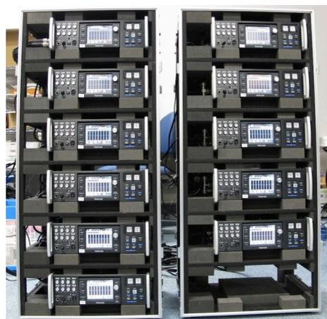
**Fig. 6:** Sound recording system based on TASCAM HS-P82. The additional one (bottom-right) recorder is used for additional recording and test signal reproduction such as swept-sine.
