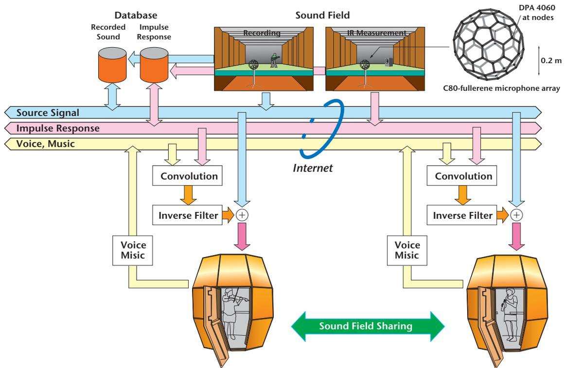
**Fig. 1:** Sound field sharing system with boundary surface control (BoSC) microphone and speaker array. The recorded signals by the C80 fullerene microphone array is re-produced in the ‘Sound Cask’ which consists of 96 channel loudspeakers after appropriate signal processing such as inverse filtering.
