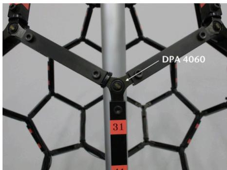
**Fig. 2:** Miniture microphone (DPA 4060) mounted at nodes of C80 fullerene structure. The #31 microphone is usually located in front.
