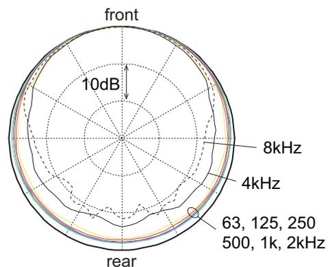
**Fig. 3:** Directivity of #31 microphone in the array. The results from 63 Hz to 8 kHz at every octave band are shown.
